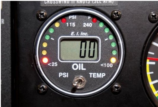
Figure 7-17 - Oil Temperature/Pressure Gauge
