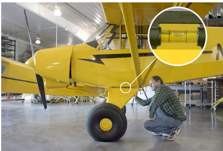
Figure 6-1 - Leveling the aircraft
