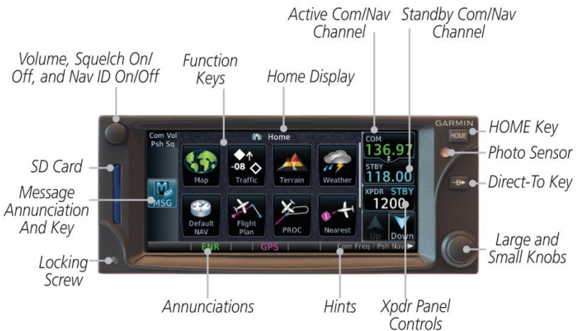
Figure 1 - GTN 635 Control and Display Layout
