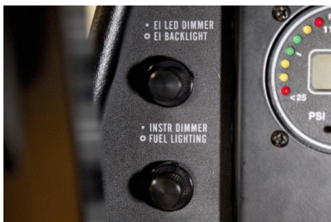
Figure 7-9 - Interior Light Dimmer Switches
